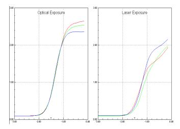
Figure 2. Sensitometric response of KODAK EKTACOLOR Edge 7 Paper to an optical exposure (left) and a laser exposure (right)
