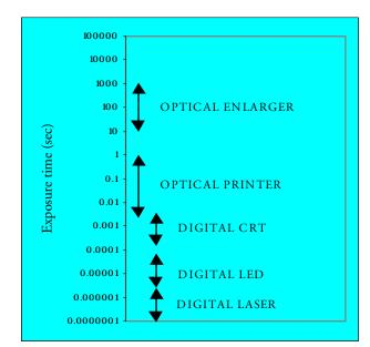
Figure 1. Pixel exposure times for optical and digital silver halide printers
