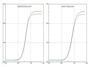
Figure 3. Sensitometric response of KODAK PROFESSIONAL Digital III paper to an optical exposure (left) and a laser exposure (right)
